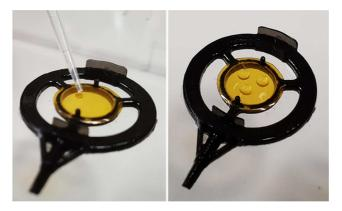
2. Flip over the sample holder and place it onto a greased cavity of a 24 well plate. The design is such that 24 sample holders will fit a 24 well plate.
