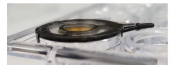
4. Ligand soaking: Remove mother liquor in a twostep procedure: – First, carefully poke a hole into the upper COC film at the appropriate position using a fine needle. The position of the puncture should be right next to the desired drop.
