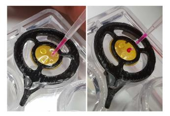
The applied solution will diffuse through the micro pores to the crystal growing side. Incubate the plate for a desired soaking time and remove the excess soaking solution with a new fine paper wick. You may soak with different compounds subsequently.
